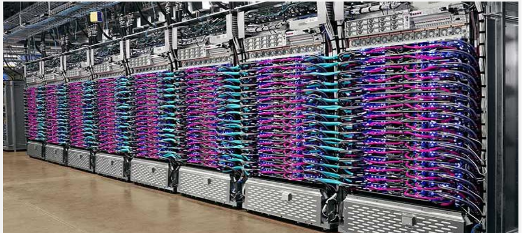
Eight-Rack Pod of Google’s Liquid-Cooled TPU Version 3 Servers for AI Workloads
